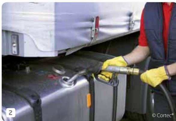
**2** Adding VpCI®-706 to diesel tanks before shipment or storage prevents the formation of corrosion.
